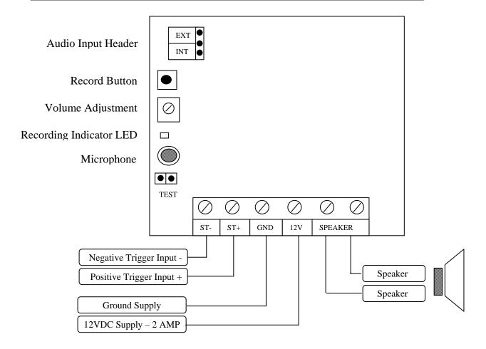
A RECORD AND PLAY BACK SYSTEM DESIGNED FOR CUSTOM MESSAGE RECORDING AND LOUD AUTOMATIC PLAY BACK. THIS MODULE IS CAPABLE OF PROVIDING 5 WATTS INTO A 4 OHM SPEAKER.
